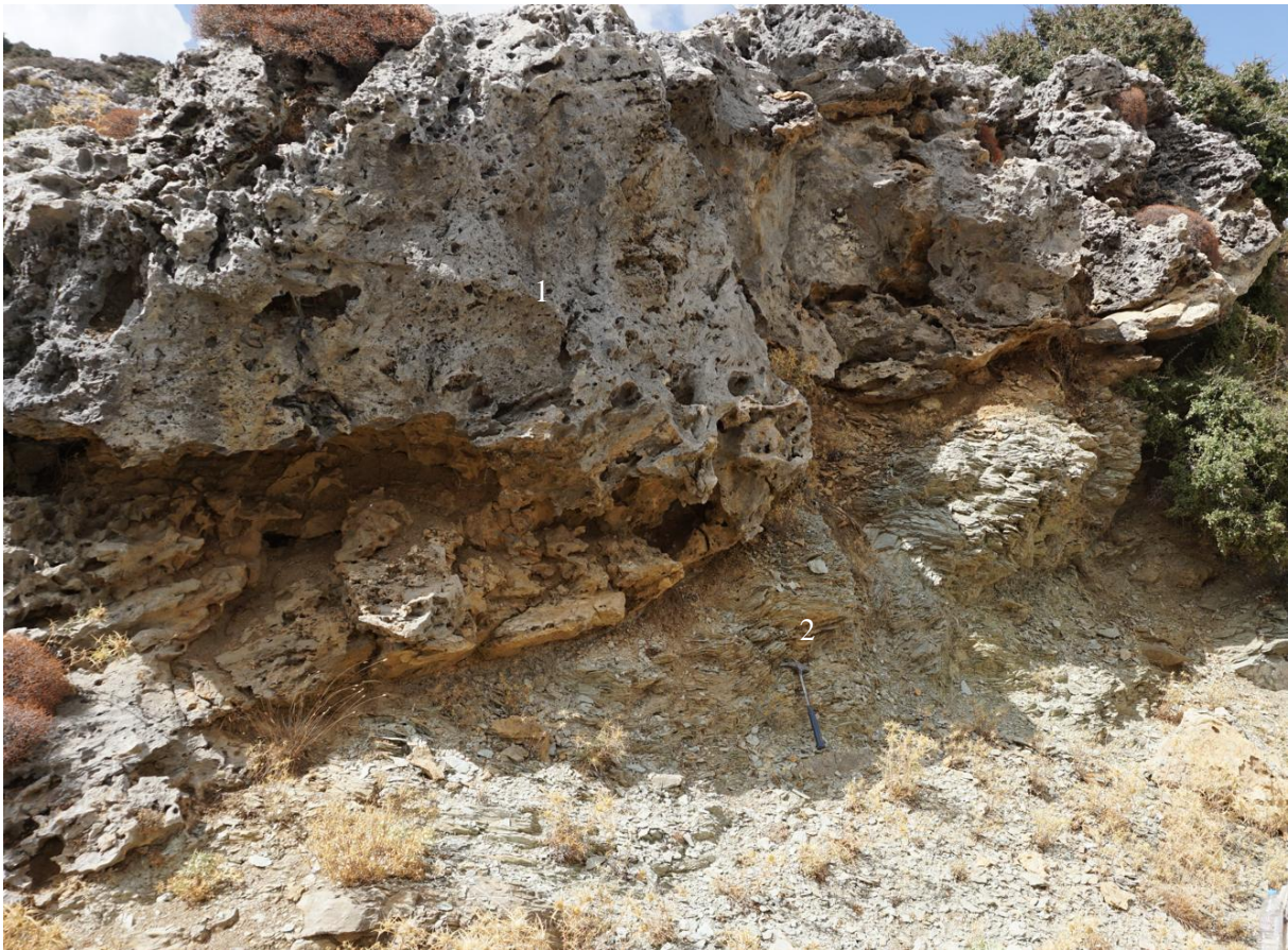
View of the fault zone. 1: Tripoliza limestone, 2: highly sheared „metaflysch“
