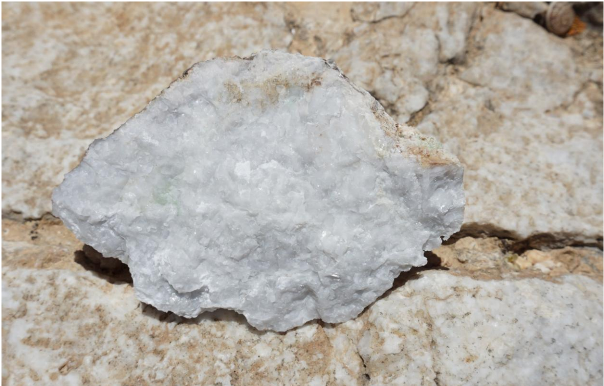
Outcrop II, Marble sample. High temperature metamorphism is indicated by the coarse-grained structure. The marble is quite white and homogeneous.
