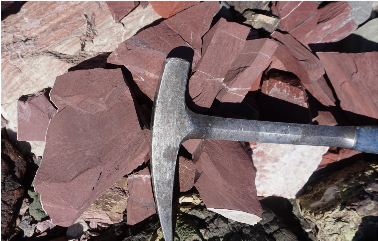
Closeup of red “slate/marl”. The slates are in reality marls as they fizz when tested with diluted hydrochloric acid.
