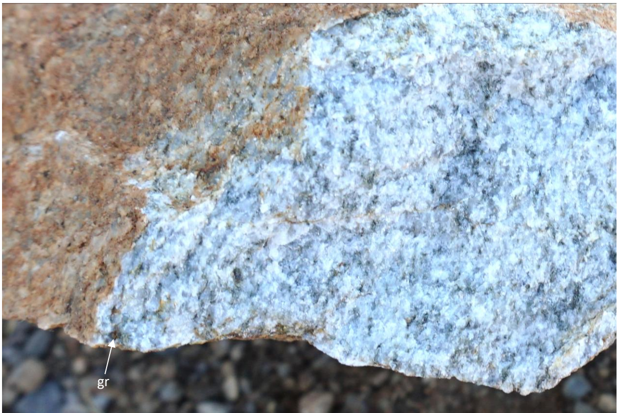
Outcrop I. Granitoid orthogneiss displaying a phanerite texture (i.e. the microstructure is made up of crystals large enough to be distinguished with the naked eye). The main minerals are quartz, feldspar and a minor content of mafic minerals such as amphiboles. This particular sample also contains a minute amount of euhedral red garnet (gr), which is normally a metamorphic mineral. According to Langosch A. et al. (2000) additional magma modification through assimilation of the country rock (paragneiss) is thought to have taken place.
