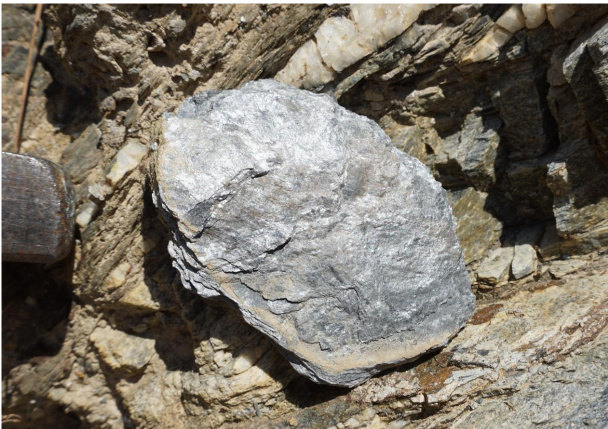
Outcrop Ia: Sample of Phyllite displaying the shiny surface typical of phyllite caused by the growth of minute muscovite and other sheet silicates at cleavage planes (left: tip of hammer)
