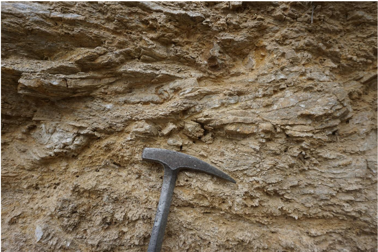
Outcrop II, highly deformed and weathered calc-silicate schist
