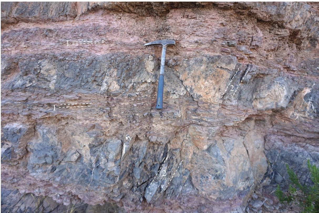
Outcrop 3, Ravdoucha Beds. Highly sheared incompetent pink shale beds (1) and highly jointed/fractured limestone beds (2).
